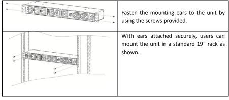
**NOTE:** If the temperature around the unit will rise above 40 °C, ventilation is required.
